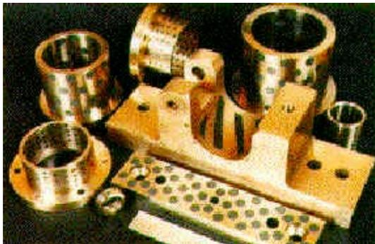
*Figure 11 – Composite self-lubricating bearings with graphite inserts are available in a wide range of shapes and sizes for applications where conventional lubrication is difficult*
