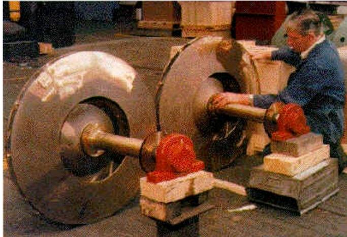
*Figure 13 –Aluminium bronze is widely used for the impellers and shafts of the blowers used to circulate these gases*
